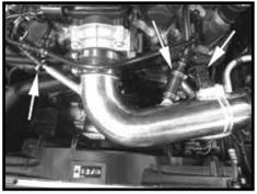
Step 14 Install the Spectre intake tube as shown and once in position tighten the clamps. Re-connect the MAFS electrical connector. Then re-connect the guick disconnect hose onto the intake tube. Re-connect the plastic vent tube to the intake tube by using the provided piece of hose and secure with the hose clamps.
