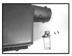
Step 8 Remove the MAFS from the factory intake.
