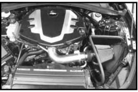
Reinstall the engine cover and secure with the factory bolt removed in step 2. Make sure that all clamps and hardware are fully tightened. Reconnect the battery cable, start the vehicle and let it warm up. Shut off and inspect the installation once more for any loose clamps, wires, or hardware. Test drive & enjoy! Your installation is now complete. Periodically check all clamps and brackets.
