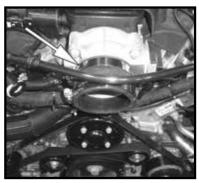
Step 13 Install the 3" coupler onto the throttle body and secure with the provided hose clamp. Install the second hose clamp onto the coupler but leave it loose for now.
