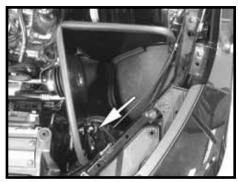
Step 12 Install the heat shield assembly into the vehicle by sliding all 3 plastic mounts into the stock air box grommets. Press firmly to make sure all 3 mounts engage fully into the grommets.
